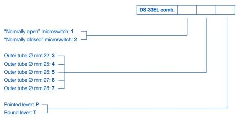
Note: Microswitch = The characteristic of the microswitch "normally open" or "normally closed" is meant with the lever leant on the knob (lowered lever).
